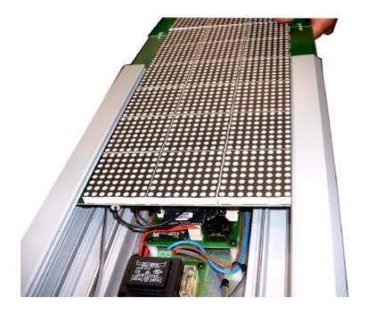
Gently ease into position both display boards and equipment tray and secure using  $2 \times No.8 \times \frac{1}{4}$  into groove between plate and extrusion.
