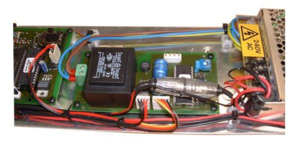
Connect to mains wire input plate. Fit IEC connector and RJ45 chassis socket ensure earth is connected.
