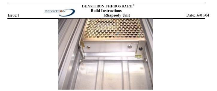
Ensure all cables and ferrites are pushed well down to avoid snagging when fitting display boards.
