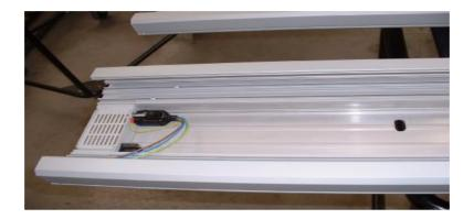
Fit the mains input end plate and rear grill to the right hand side of the unit.
