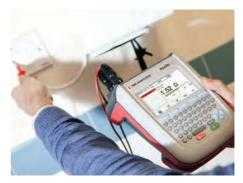
Fixed equipment or appliances are more difficult to inspect and test due to their connection to the fixed wiring of an installation. This does not mean that only visual inspections are required for these types of
