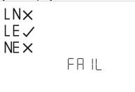
In the event of a test failure, disconnect the PrimeTest 100 from the supply and rectify the fault.
