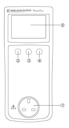
Figure 1. PrimeTest 100 Front View
